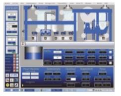
project can be controlled with just one monitor. An added bonus of the zenOn monitor management tool is the relative picture call-up: The picture is displayed on the monitor on which it is called up. Furthermore, the monitor on which the picture is to be displayed can also be exclusively defined. In addition, during runtime, a monitor selection can be shown with which the user can select on which monitor the picture is to be displayed.
